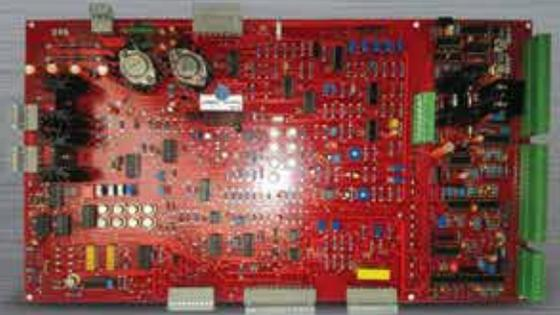
MAIN LOGIC CONTROL BOARD FOR MELTING FURNACES WITH POWER UP TO 1000KW AND FREQUENCY RANGE UP TO 10,000 HERTZ
